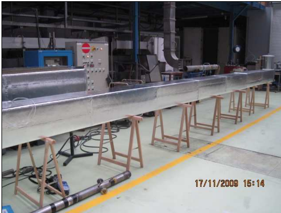
Figure 8 : View of the airtightness test plant
