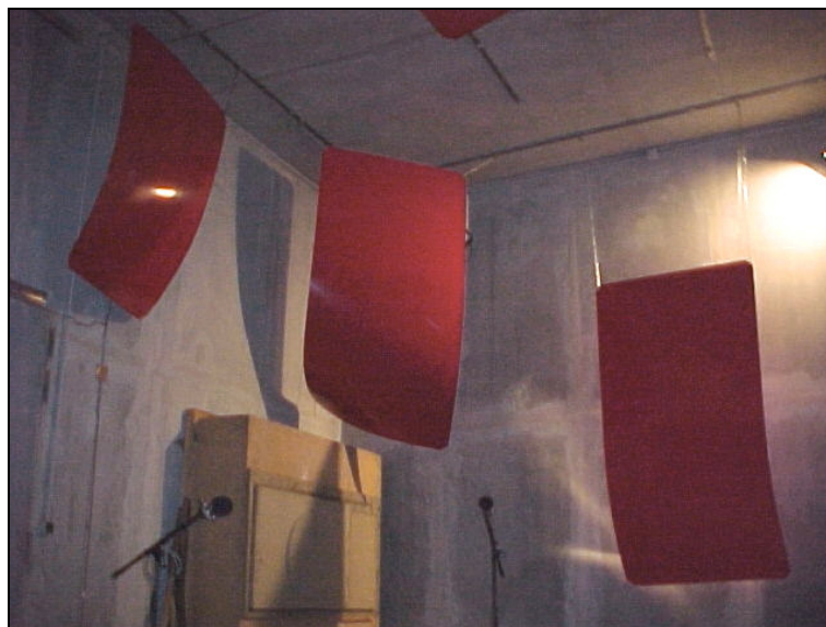
Figure 15 : View of the testing chamber with diffusers
